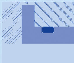
Clamping flange with additional O-ring seal.
